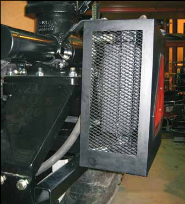
Oil cooler. In warm conditions, operating a harvester head or a felling grapple, is an oil cooler needed
