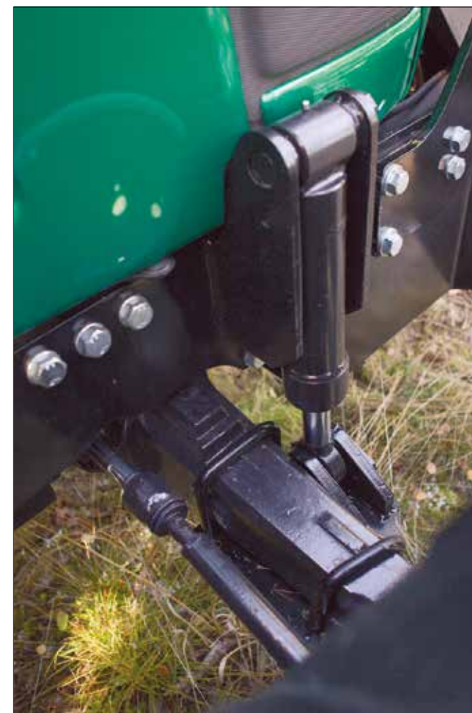
Front axle locking unit set for Valtra tractors without air-suspended axle. Set consists of two cylinders, hoses and valve.
