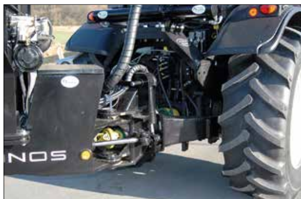
Y-tractor axle drawbar with hydraulic locking and frame steering (with 2 cylinders)
